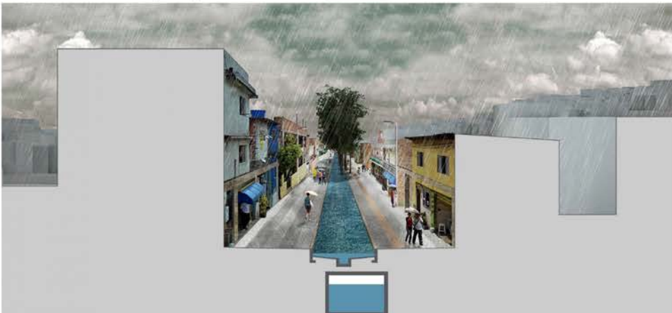
The canal when it rains is helped by a subterranean system
