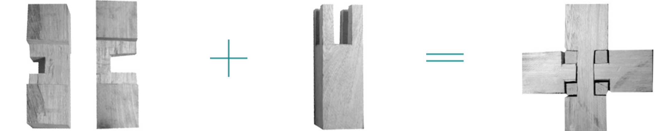
Connection Joint Detail 02 (Physical Model at 1:1)
